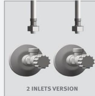
**MAKE SURE THAT THE FILTERS ARE INSTALLED BETWEEN THE FLEXIBLE PIPE AND THE SHUT OFF VALVE/ANGLE VALVE (NOT SUPPLIED).**
